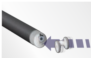
1. Install Packer's Wheel Assembly
