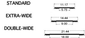
RUBBER • The Seal is supplied in either EPDIM or Nitrile. The EPDM is used in applications for potable water, wastewater, and sea/brackish water. The Nitrile seal provides superior resistance to gas, oil, and petroleum-based reagents making it ideal for natural gas applications.
